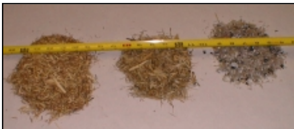
Figure 6.—Raw Material Components (l-r) — Slivers, Flakes, and Ground Plastic Film.
